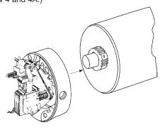
6 Mount brake endplate to motor C-face.
