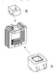
A) Reinsert plunger into coil; drop pivot pin into cradle of support plate.
