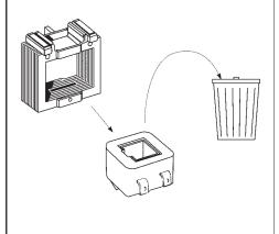
A) Insert new coil. (Lead wires in same position as old coil.)
