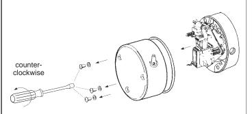
Slide endplate over hub noting position of stabilizer springs, if used. (Refer to Friction Disc Replacement, View 4 and 4A.)
