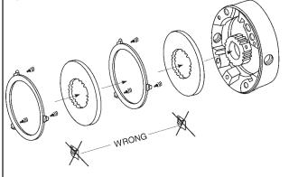
Reposition support plate on endplate and tighten mounting screws to 55 lb-in.
