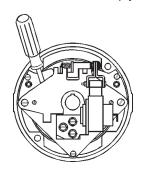
Lift plunger/solenoid lever assembly out of coil.
