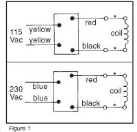
\* Clutch coil lead wires are black.
